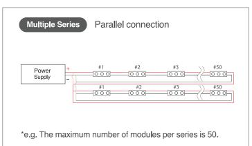
If you require **multiple modules**, they must be wired in parallel as a safe electrical operation mode. **Serial connection is not recommended**, as unbalanced voltage drops can lead to hazardous overload, potentially damaging the LED modules and causing uneven brightness
