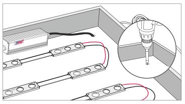
6 Drill holes along the edge of the channel letter or lightbox connect to the power supply
