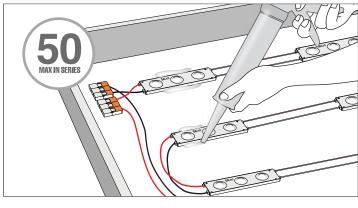
**4** WAGO connectors enable quick wiring of LEDs in series. Secure LEDs with silicone glue.
