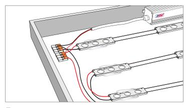
Wire both ends of LED modules to the power supply (refer to page 3). For multiple series, connect them in parallel to avoid voltage drop and ensure even brightness.
