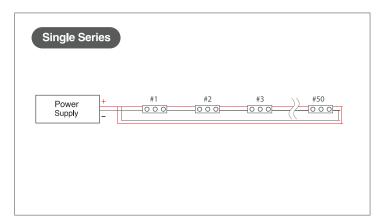
Do not exceed the maximum number of LED modules per series (refer to each item's spec sheet for specific numbers). We recommend wiring both ends of LED modules to the power supply.
