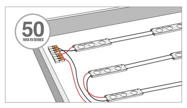
**3** Ensure modules are connected in series or parallel (refer to Figure 2 on page 3). Avoid exceeding the maximum module count to prevent voltage drops.
